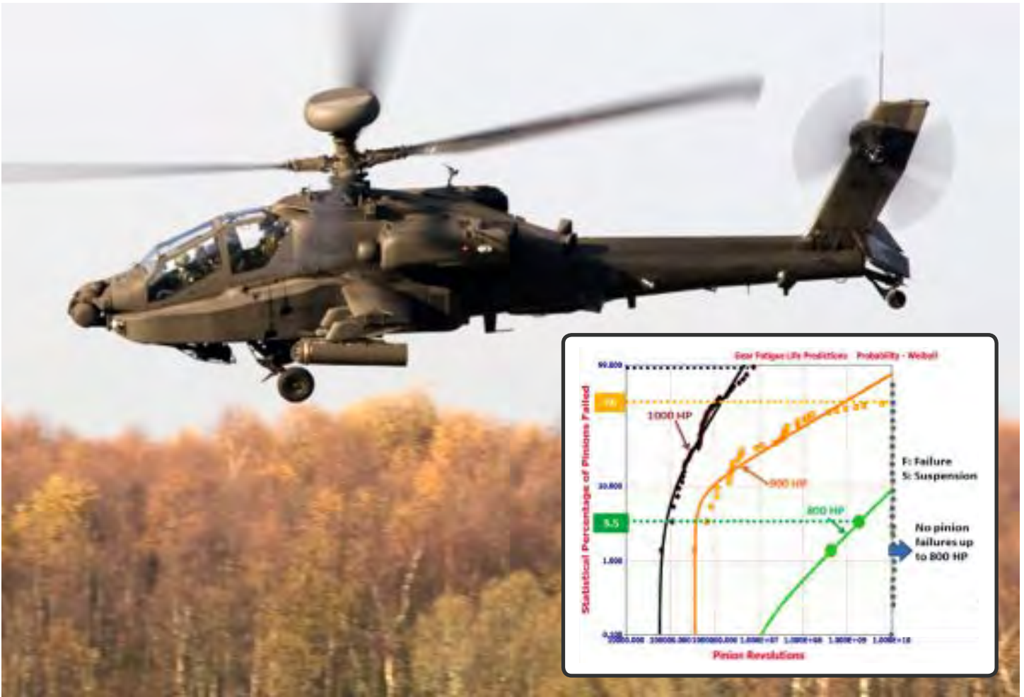
Using prognostic models, a design team can examine the overload testing and performance limits of a drive system before beginning physical testing.
