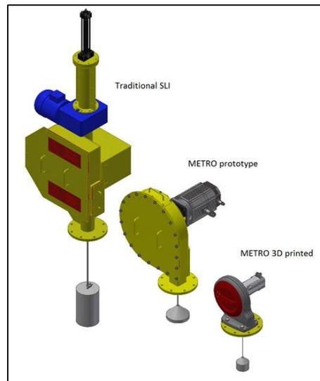
Figure 5 - From traditional shaft level indicator to 3D Printed METRO
