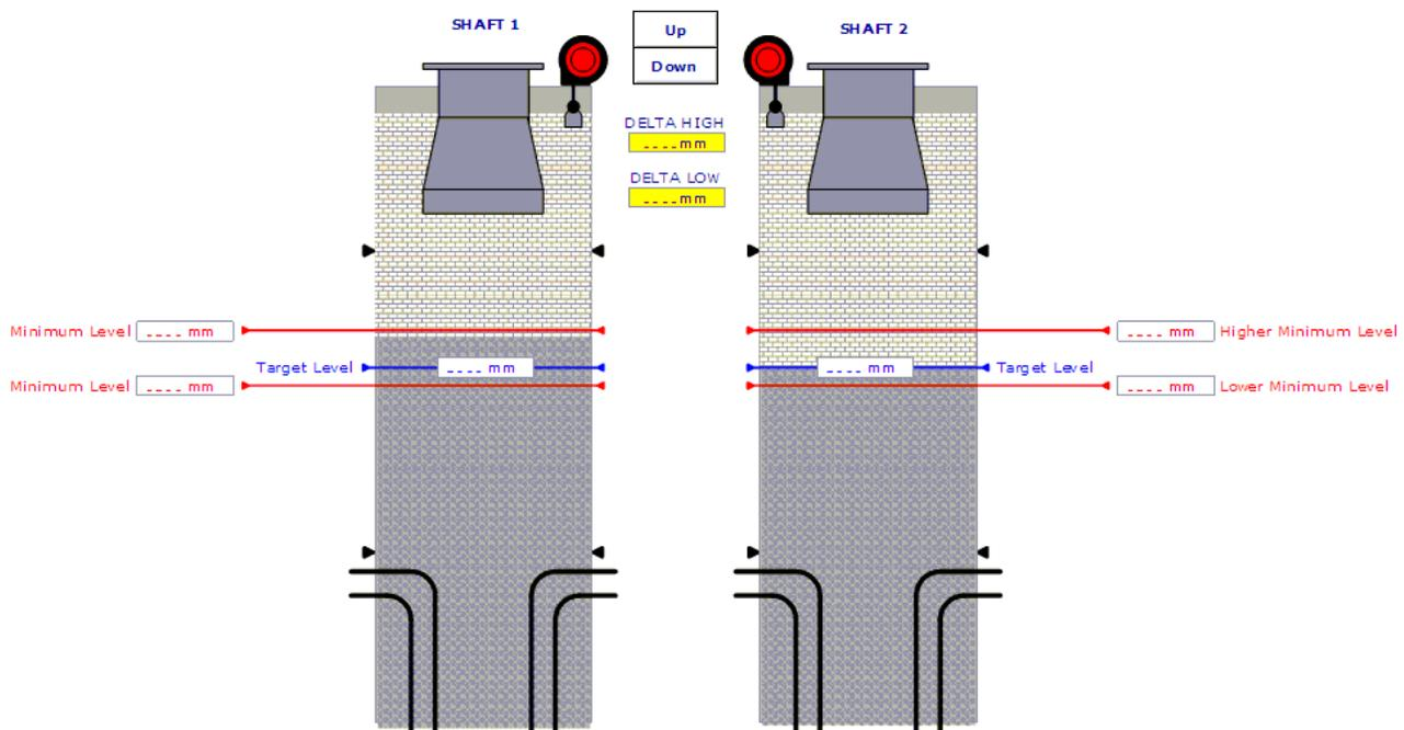
Figure 1 Kiln level representation in a vertical PFR Kiln
