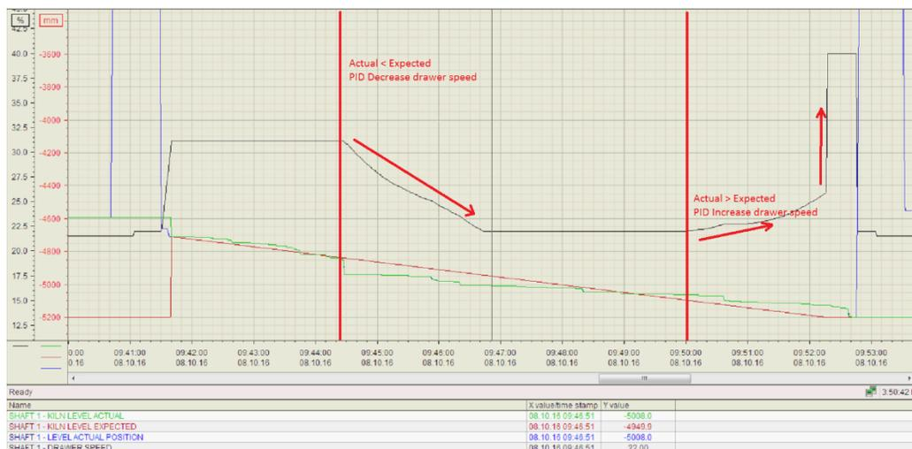
Figure 4 Typical discharge system PID cycle
