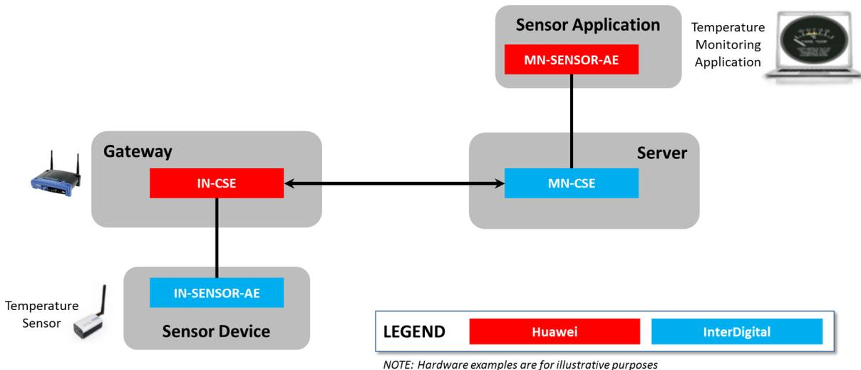
Figure 2 Example test-case: prepare a sensor to publish data to a subscriber application
