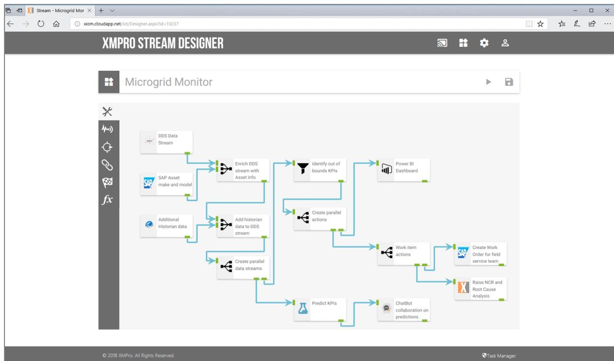
Figure 8 - Example of an event stream that integrates IoT data into operational workflows
