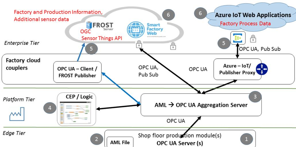
Figure 4: 3 Tier Architecture for Factory Integration. Abbreviations AML: AutomationML, CEP: Complex Event Processing, OGC: Open Geospatial Consortium, FROST: Fraunhofer Open Source SensorThings API Server
