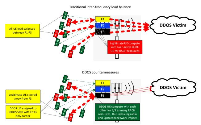
Figure 4-5: Inter-frequency load balance for covert DDoS countermeasures.
