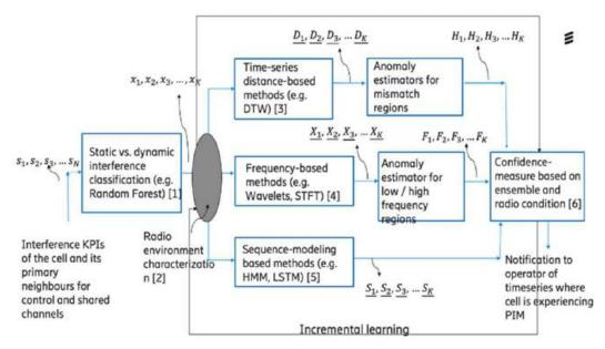
Figure 3-2: Block-diagram of the ensemble-based approach for time series ensemble-based approach for network anomaly detection under DoS attacks.
