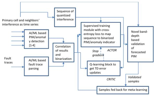
Figure 3-3: Block diagram of the self-supervised approach for anomaly detection from uplink noise rise.
