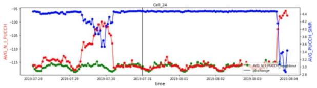
Figure 3-1: Rise in Uplink noise due to DoS may not have an impact on the neighboring cells. In blue is SINR of primary cell, and in red the interference of primary cell. In green, is shown the interference of the first neighbor.
