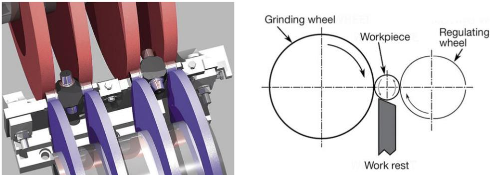
Figure 7: Centerless Grinding
