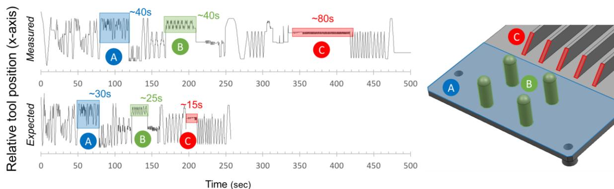
Figure 3: Comparison of simulated data for part build generated by Mastercam compared to actual machine data. Note: The X-position of each dataset has been translated for ease of comparison. The vertical scales are consistent with both datasets.
