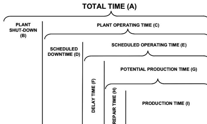
Figure 5: Chart of Equipment Availability Parameters
