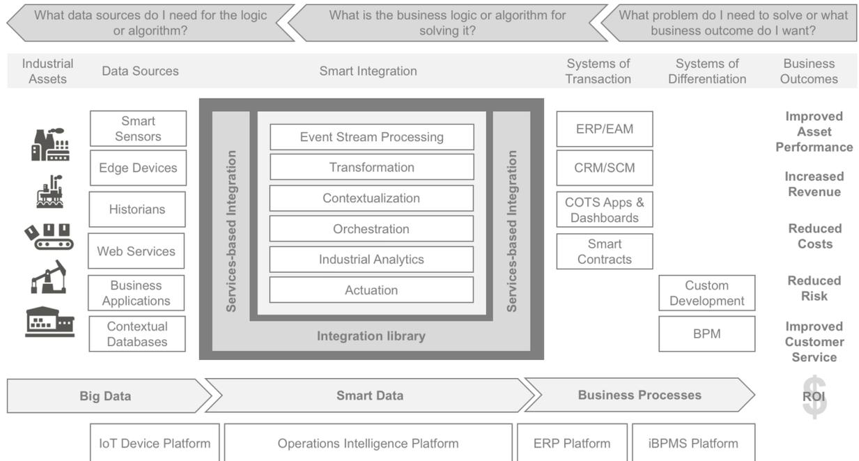
Figure 2 - I2OC (IoT to Operational Capability) framework
