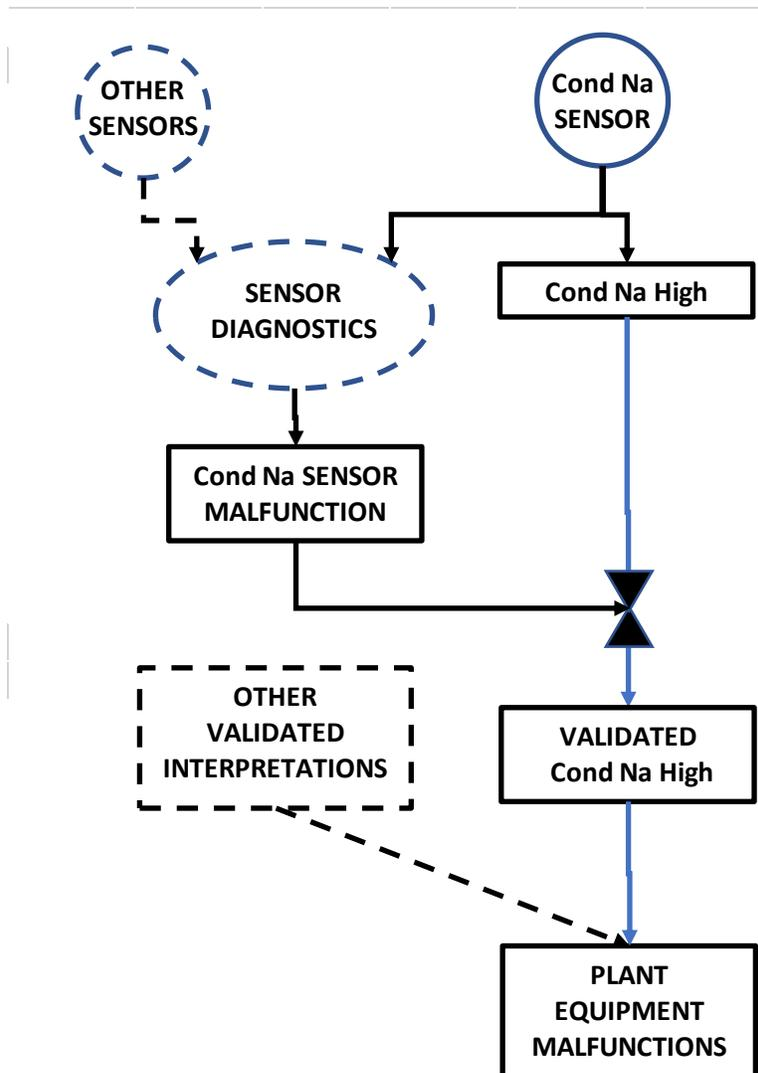
Figure 4: Schematic of diagnosis using the Condensate sodium sensor, showing sensor diagnosis and the method of using a Paralt rule to reduce confidence in the validated Condensate sodium high. Dotted shapes and lines are used to represent many hypotheses and rules.
