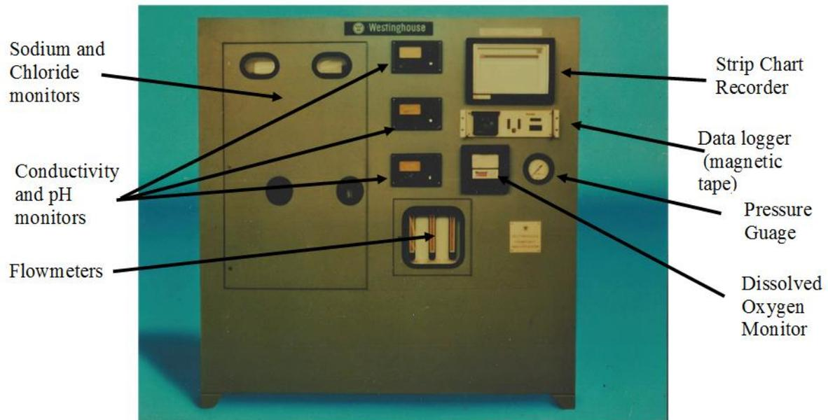
Figure 3: Westinghouse Steam Purity Analyzer System, ca. 1981. The box was about 5 feet high.
