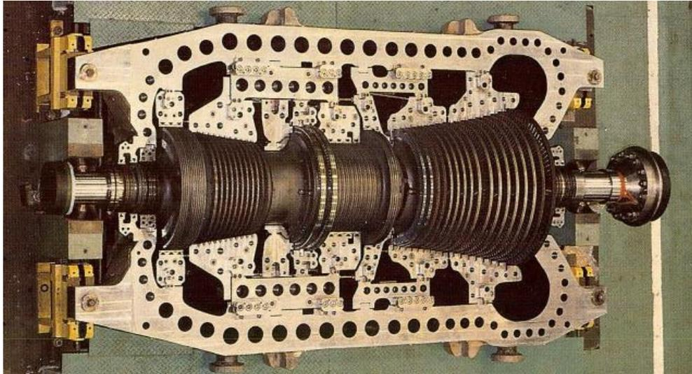
*Figure 2: Combined High-Pressure and Intermediate-Pressure steam turbines, ca 1985. As the steam expands, the turbine blades become longer. At the end of the Low-Pressure turbine, they were typically 31 inches long.<sup>1</sup>*
