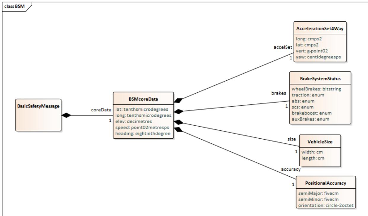
Figure 5: Physical Data Model for BSM
