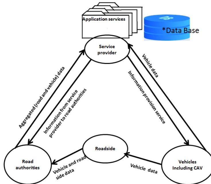
Figure 1: The conceptual framework of a vehicle probe system
