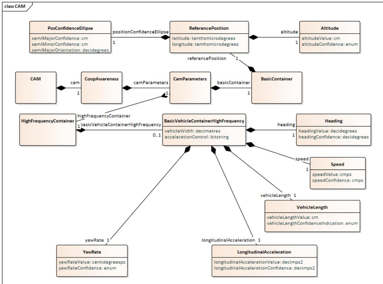
Figure 4: Physical Data Model for CAM
