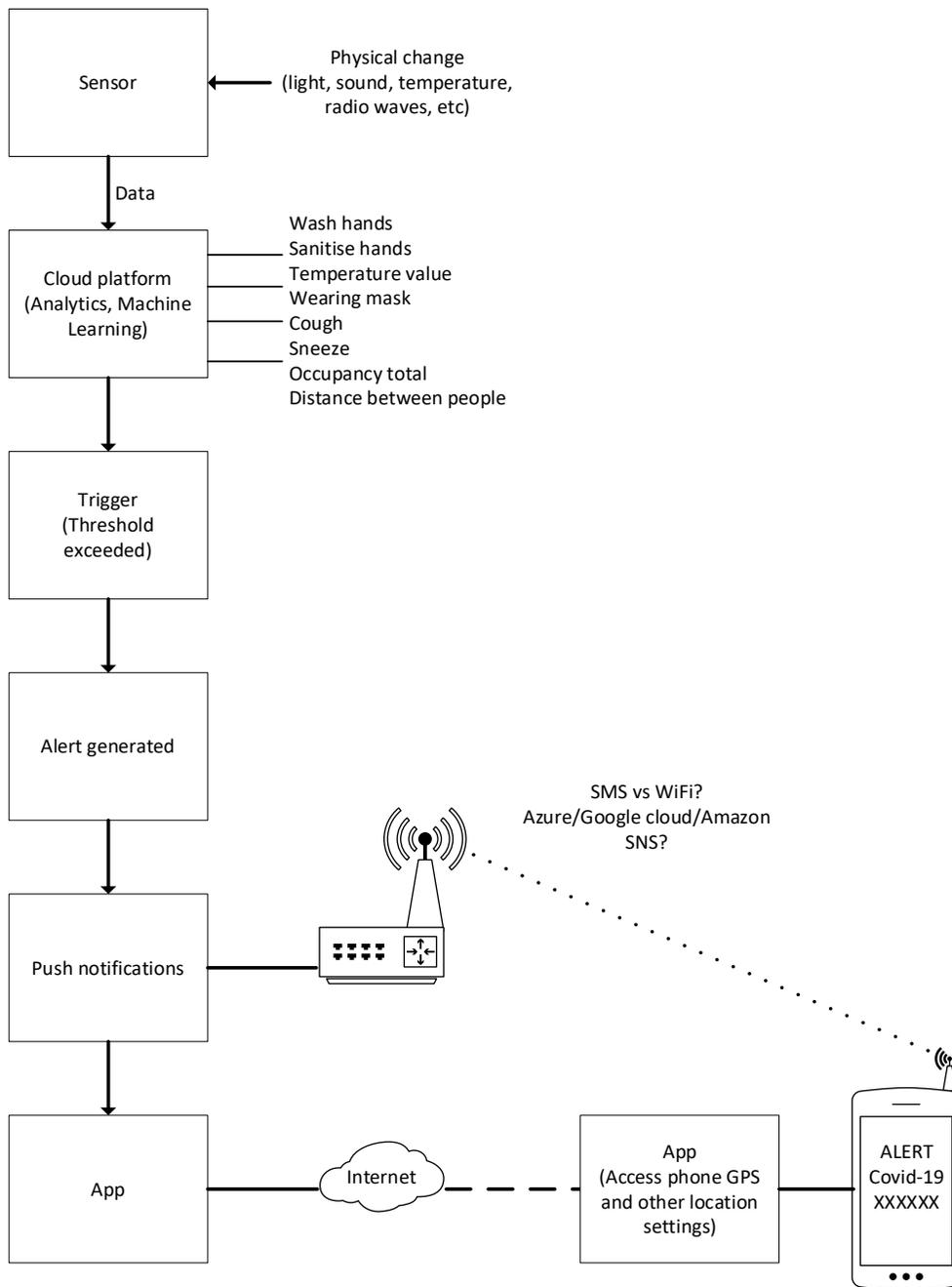
Fig. 14: Conceptual Framework of IoT based Alert System
