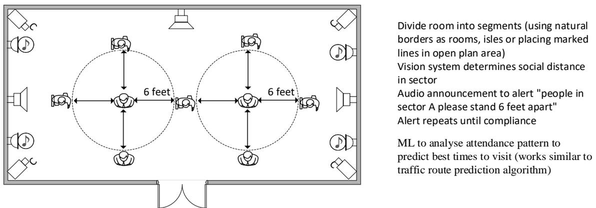
Fig. 13: IoT sensors – Internal mounted camera, microphone and speakers
