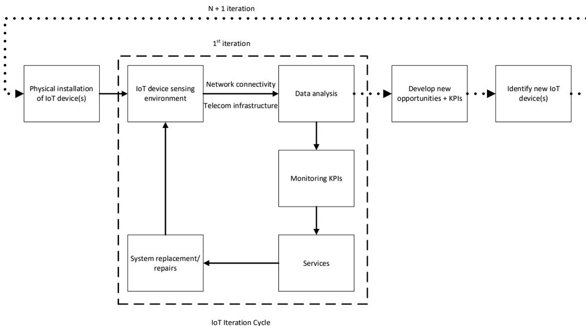
*Fig. 16: IoT Iteration Cycle*
