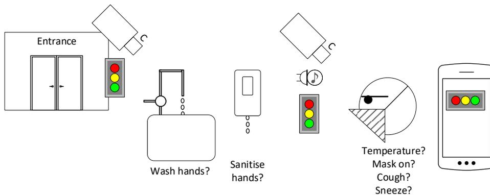
Fig. 12: IoT sensors - External mounted camera, microphone and status indicator
