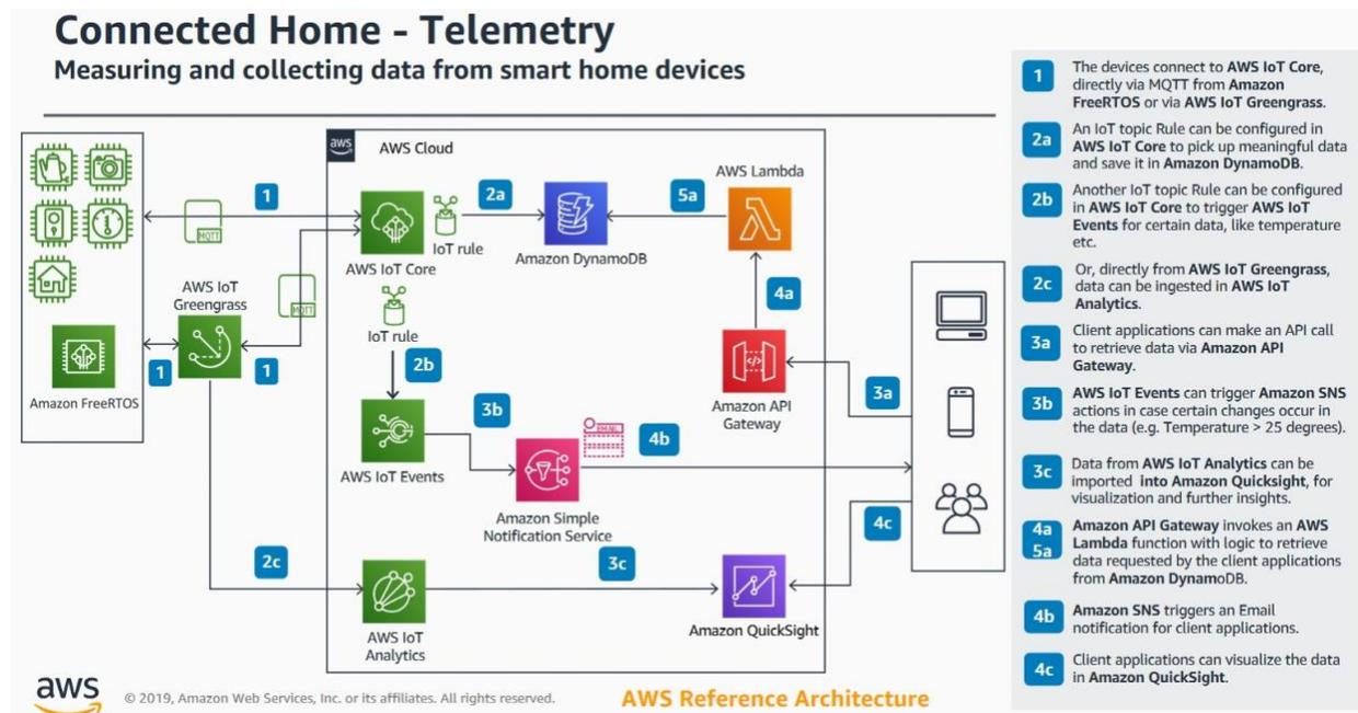
Fig. 15: AWS Telemetry Architecture<sup>64</sup>
