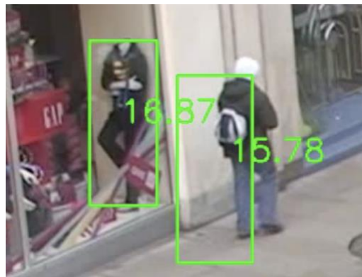
Fig. 13: A mannequin being detected as a person standing at ~16 meters from camera
