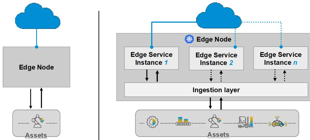
*Fig. 5 - High Availability for Edge Computing (left: single edge node configuration; right: high-availability edge node configuration).*
