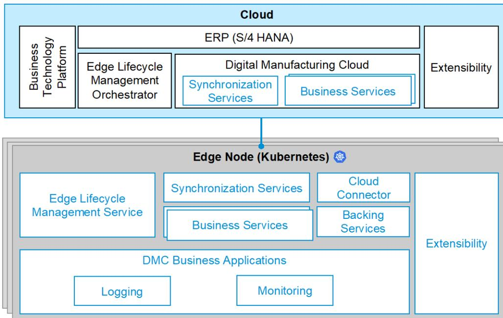
Fig. 4 - Edge computing architecture for mission critical execution of distributed manufacturing processes on the edge [20] [21].
