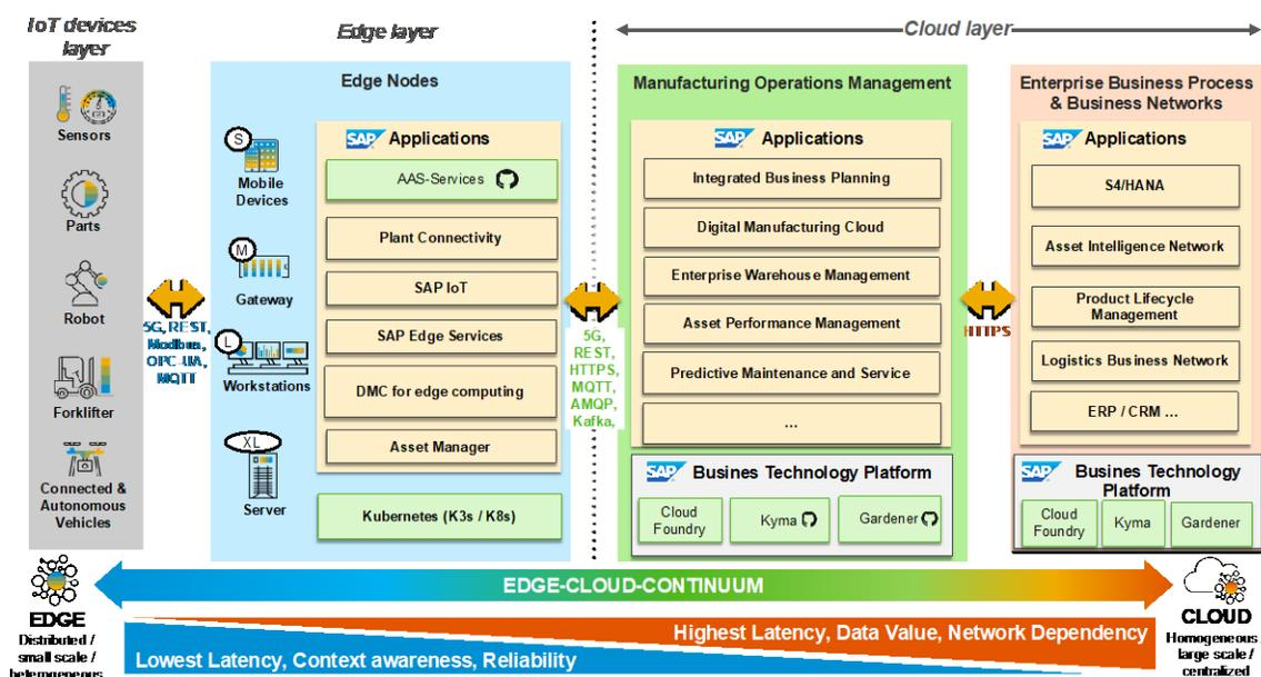
Fig. 2 - Edge-cloud continuum for enabling mission critical execution of distributed manufacturing processes
