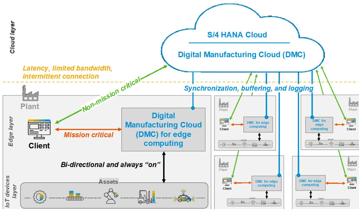
Fig. 3 - Approach for ensuring business continuity for mission critical applications based on [14].
