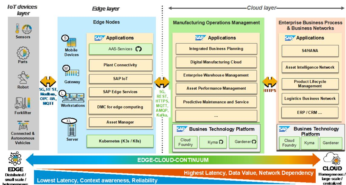
Fig. 2 - Edge-cloud continuum for enabling mission critical execution of distributed manufacturing processes
