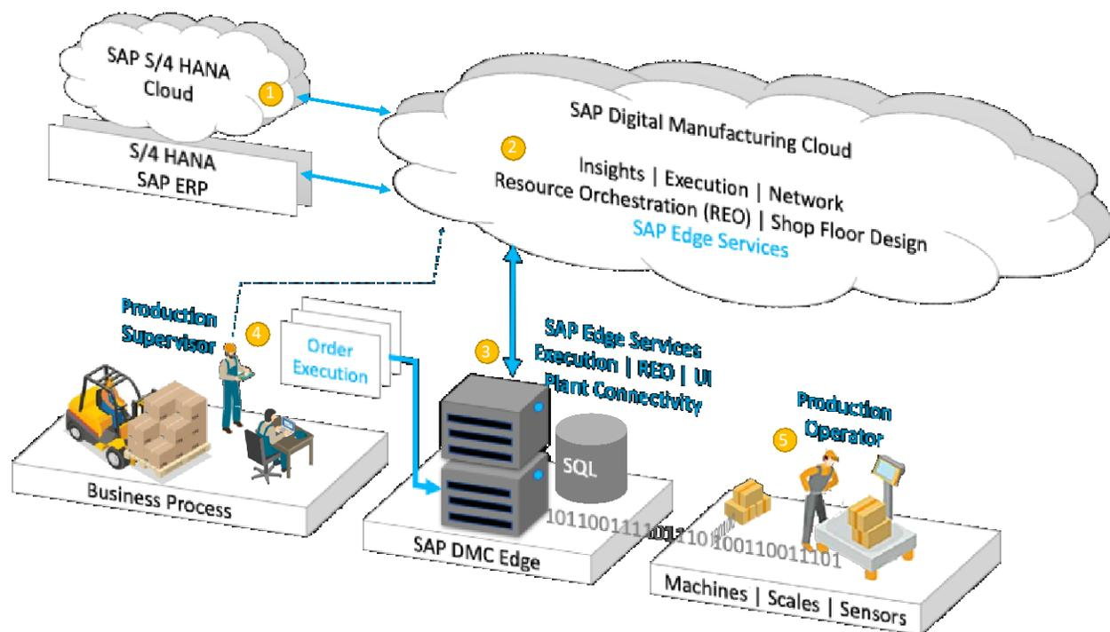
Fig. 7 - Scenario of mission critical manufacturing process using SAP's edge computing solutions.
