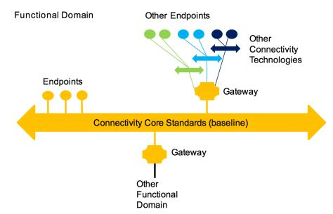
*Connectivity Gateway Concept*. Gateways integrate other connectivity technologies used within a functional domain and interface with connectivity core standards in other functional domains.
