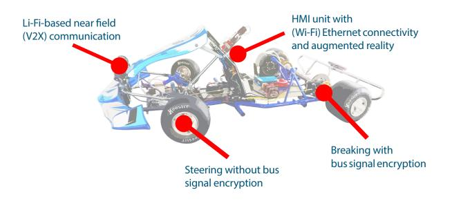
The idea is to start with a few features and build it out over time. The closer the Go-Kart is to a fully functional auto, the better the OTA features can be demonstrated. The Testbed is far from complete; Power is not yet connected and there are not any mobile network connections such as GSM or better. The cloud connectivity is currently to an AWS server and provides the following services:
