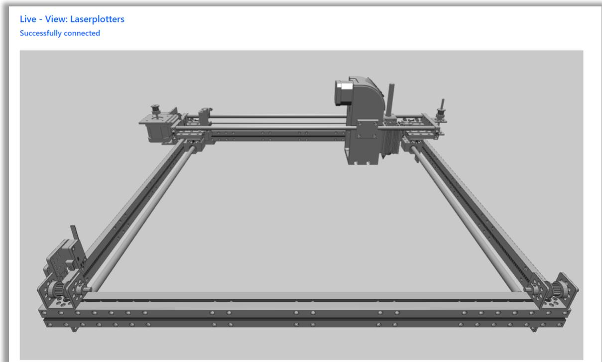
*Fig. 11: Live view of the up-to-date state of the asset. The animation is moving accordingly to the current position variables in the OPC UA server. The model is stripped down to the essentials to speed up the animation.*
