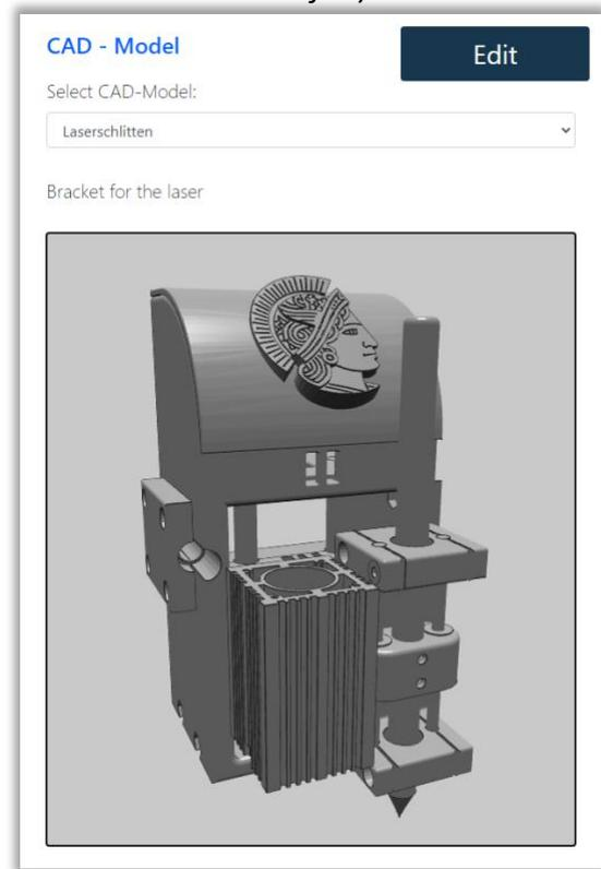
Fig. 10: Visualization of 3D geometry of a laser plotter component.
