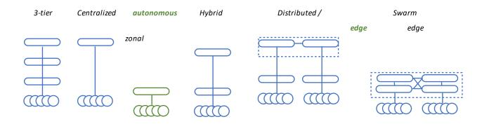
In those diagrams, rounds represent things which can be sensors, controllers. The rectangular objects represent levels/nodes of data handling and/or storage.
