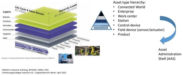
Figure\_Apx 5: Reference Architecture Model Industrie 4.0 (RAMI4.0)
