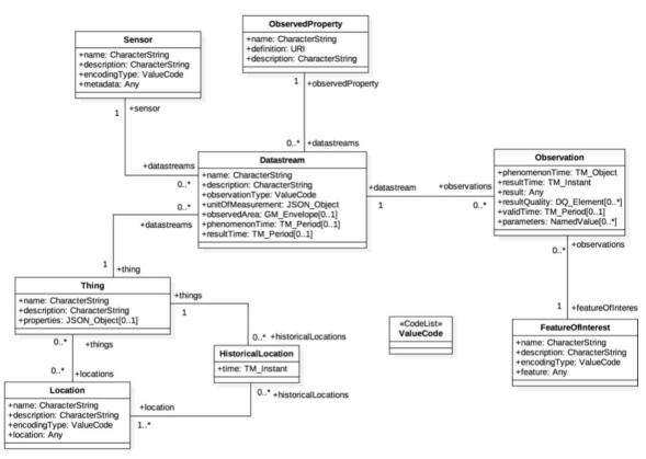
Figure\_Apx 3: Sensing Entities in SensorThingsAPI Part 1
