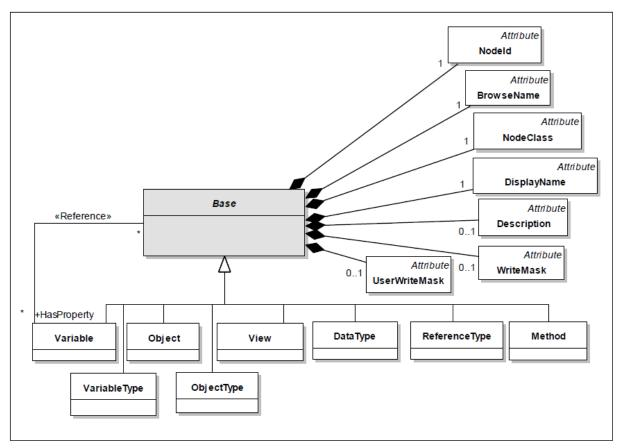
Figure\_Apx 9: Base metamodel of Nodes (OPC UA Part 3, Fig. B.4)
