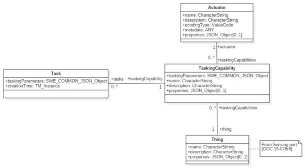
Figure\_Apx 4: Tasking Entities in SensorThingsAPI Part 2
