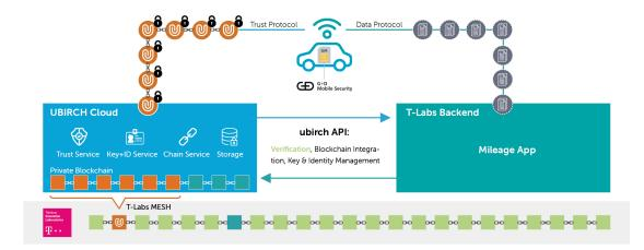
The car produces two data streams for its IoT data, the data protocol and the trust protocol created directly on the SIM. While the data protocol can be handled by the Mileage App Backend, the trust protocol is handled by the UBIRCH cloud, anchoring the trust protocol packages into the blockchain using T-Labs Stax service. Whenever needed within the business case, the IoT data can be verified for its authenticity against the blockchain using the UBIRCH API.
