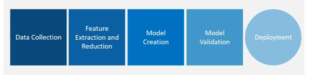
Figure 6-3 Workflow for developing analytic models
