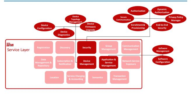
Figure 6 Illustrative Features of oneM2M Common Service Layer Functions (Source: oneM2M)
