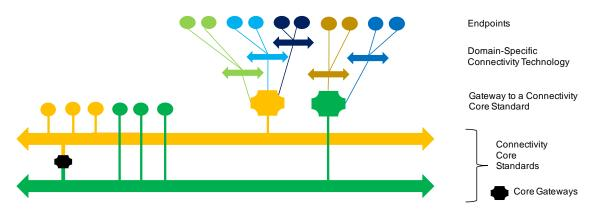
Figure 10 Standardized gateway for end-point interoperability (Source: IIC IICF)
