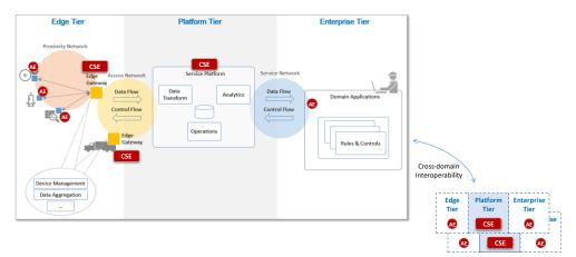
Figure 8 IIRA 3-tier architecture pattern mapping to oneM2M architecture elements
