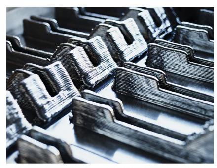
A bed of additive-manufactured titanium components for the Boeing 787 Dreamliner. Photo via Norsk Titanium.
