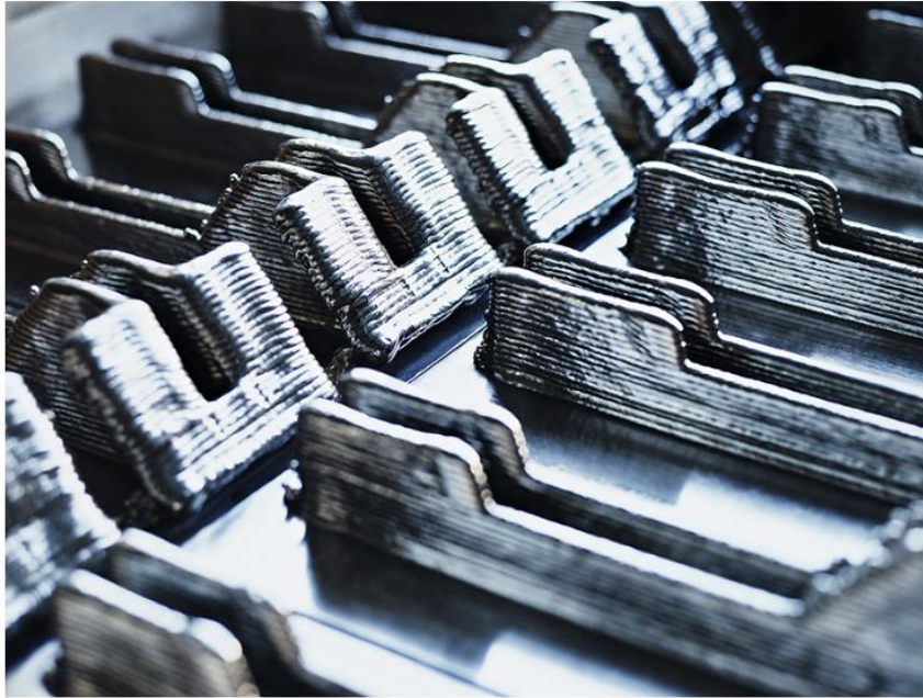
A bed of additive-manufactured titanium components for the Boeing 787 Dreamliner. Photo via Norsk Titanium.
