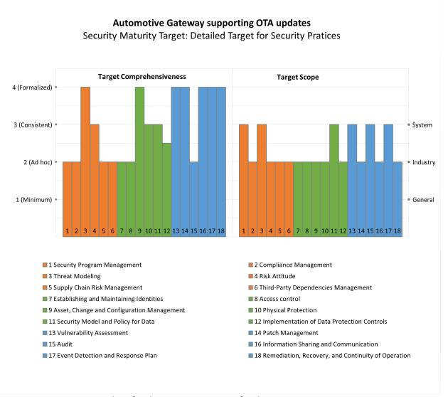
Figure 13-3: Target values for the Security Practices for the Automotive Gateway Supporting OTA Updates case study
