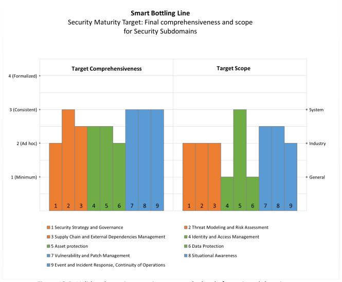
Figure 12-5: Validated security maturity target at the level of security subdomains
