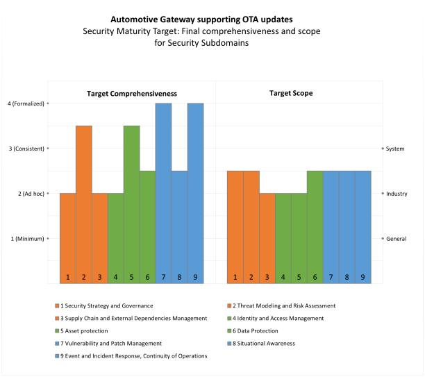
Figure 13-5: Validated security maturity target at the level of security subdomains for the Automotive Gateway Supporting OTA Updates case study
