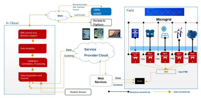
Figure 2: Deployed communication and control tiered architecture for microgrid and distribution grid management
