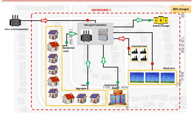
Figure 4: Microgrid Operator management interface allows field device monitoring and management
