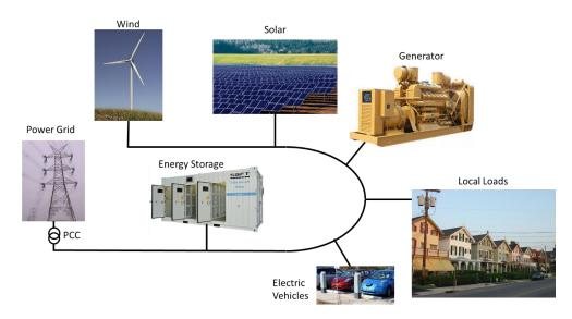
Figure 1: Example of a microgrid that uses data communication and edge intelligence to automate local power generation and balance against the power load. Microgrids help to integrate intermittent energy sources such as solar and wind.
